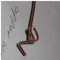
Figure L: Bend the end of the wire into this shape to fit into the rose
