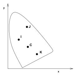
In the CIE diagram above, **C** is the point of equal energy where  $x = y = z = \frac{1}{3}$ . (Note that conventionally the CIE diagram only shows the x and y axes).
