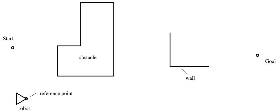
(a) Draw how the obstacles should be grown in order to reduce the path planning problem for the robot to that of finding a collision free path for a point through a field of obstacles. Assume the robot is unable to rotate in its motion, it can only translate. (3)
