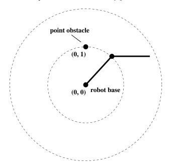
The base of the robot is located at (0,0), both links have a length of 1 and the joints have no limits on their rotation. A point obstacle is located in the workspace at (0,1).
