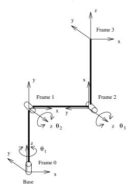
(a) Write the 4x4 homogeneous transformation matrices describing Frames 1, 2 and 3 in terms of Frame 0.
