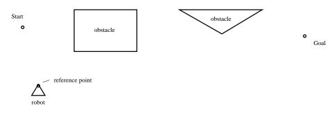
(a) Draw how the obstacles should be grown in order to reduce the path planning problem for the robot to that of finding a collision free path for a point through a field of obstacles. Assume the robot is unable to rotate in its motion, it can only translate.
