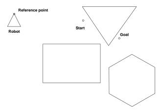
(a) Assuming a **point** robot, draw the visibility graph of the paths between the robot start state to its goal state. Highlight the optimal (shortest) path.
