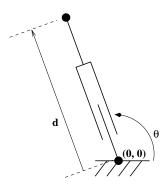
(a) Write out the  $2 \times 2$  Jacobian matrix relating the velocity of the end effector in x and y to the joint velocities  $\dot{\theta}$  and  $\dot{d}$ . Each element of the Jacobian should be expressed in terms of the robot's current configuration  $(\theta, d)$ .
