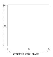
(a) Assume that the robot's movements are restricted to allow only the following configurations:  $\theta_1 \in [\pi, 2\pi]$  and  $\theta_2 \in [0, 2\pi]$ . Draw a diagram showing the robot's physical workspace.
