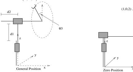
Work out the forward kinematics for this robot.
