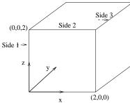
A base coordinate frame is placed at the origin, and travels along the edges of the cube by going up side 1, along side 2 and out along side 3. At each corner, the frame is rotated by  $90^{\circ}$  so that the next transition is along the current z-axis.
